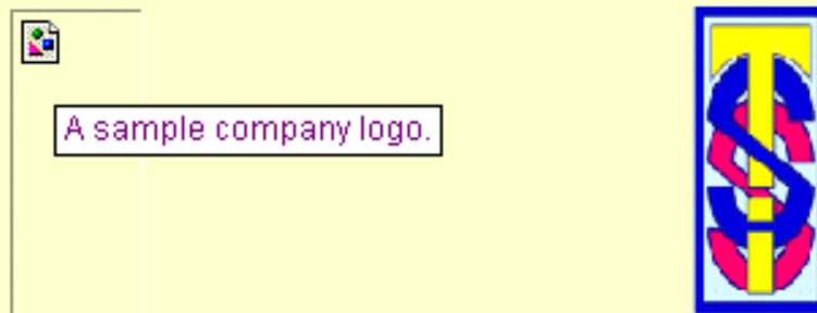
Figure 19.01. The IMG tag for this file includes the element ALT="A sample company logo." The ALT
