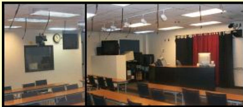
Figure 20.08. Distance Learning Classroom at UNL. Typically used for satellite or in-state network television, this room was equipped to accommodate Internet 2 (4 Mbit) television, both in and out. Left view: control room, with video camera above window. Right view: instructor podium, monitors for viewing from other sharing sites, camera. The dark rod-like objects hanging from the ceiling throughout the room are microphones.
