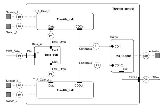
Fig. 2. Revised proposal for the Throttle Control System decomposition
