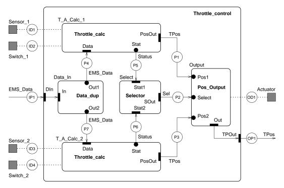
Fig. 1. Initial proposal for the Throttle Control System decomposition
