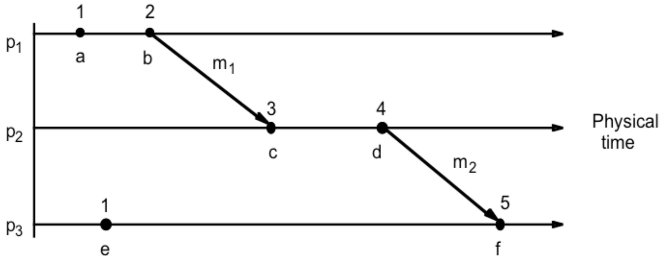
**LC1:**  $L_i$  is incremented *before* each event is issued at process  $p_i$ :  $L_i := L_i + 1$ .
