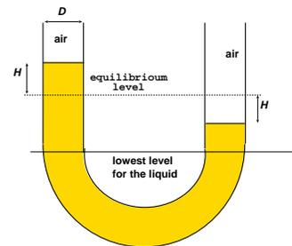
Fig. -7.5. Flow in an oscillating manometer.
