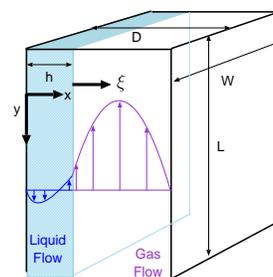
Fig. -10.15. A diagram to explain the flood in a two dimension geometry.
