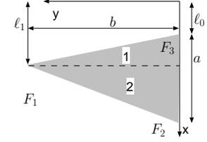
Fig. -4.23. The general forces acting on a non symmetrical straight area.
