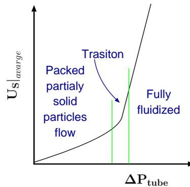
Fig. -10.8. The terminal velocity that left the solid particles.
