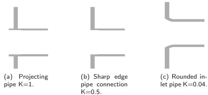
Fig. -7.4. Typical resistance for selected outlet configuration.
