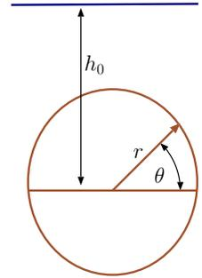
Fig. -4.34. The floating forces on Immersed Cylinder.
