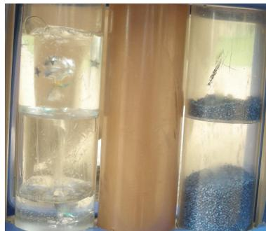
Fig. -10.12. Picture of Counter-current flow in liquid-gas and solid-gas configurations. The container is made of two compartments. The upper compartment is filled with the heavy phase (liquid, water solution, or small wood particles) by rotating the container. Even though the solid-gas ratio is smaller, it can be noticed that the solid-gas is faster than the liquid-gas flow.
