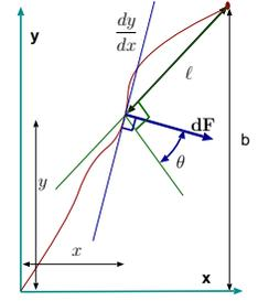
Fig. -4.32. The difference between the slop and the direction angle.
