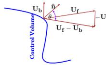
Fig. -5.3. Schematics of velocities at the interface.
