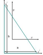
Fig. -3.13. Product of inertia for triangle.
