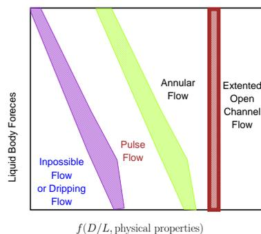
Fig. -10.10. Counter-flow in vertical tubes map.
