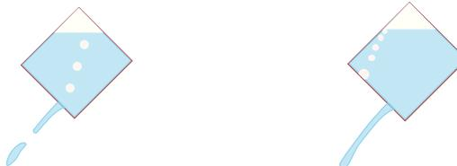
Fig. -10.11. Counter-current flow in a can (the left figure) has only one hole thus pulse flow and a flow with two holes (right picture).
