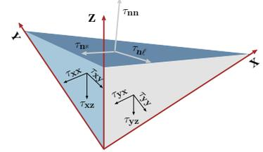
Fig. -8.5. Stress diagram on a tetrahedron shape.
