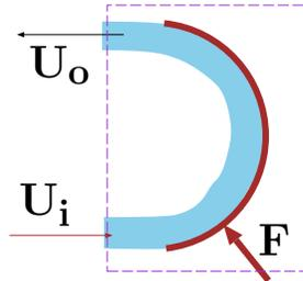
Fig b. Schematics of maximum angle for impinged by a jet.
