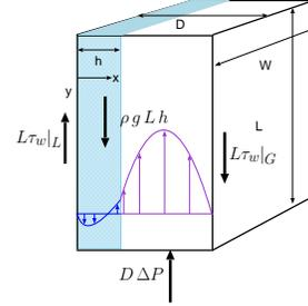
Fig. -10.16. General forces diagram to calculated the in a two dimension geometry.
