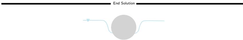
Fig. -4.46. A heavy needle is floating on a liquid.
