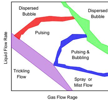
Fig. -10.7. A dimensional vertical flow map under very low gravity against the gravity.
