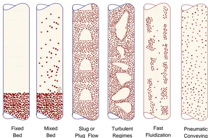
Fig. -10.9. The flow patterns in solid-liquid flow.
