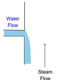
Fig. -10.13. Flood in vertical pipe.
