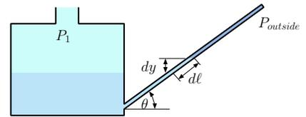
$$P_1 - P_{outside} = \rho g dl \quad \text{Fig. -4.8. Inclined manometer.} \quad (4.25)$$
