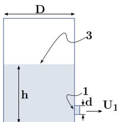
Fig. -7.8. Tank control volume for Example 7.2.
