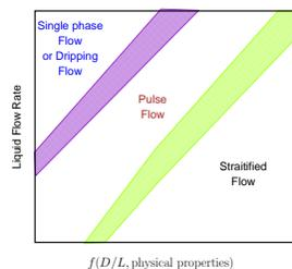
Fig. -10.14. A flow map to explain the horizontal counter-current flow.
