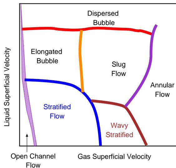
Fig. -10.5. Modified Mandhane map for flow regime in horizontal tubes.
