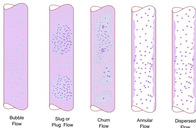
Fig. -10.6. Gas and liquid in Flow in vertical tube against the gravity.
