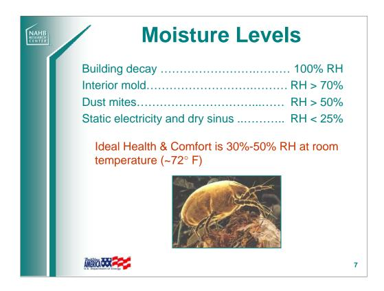
Liquid water (a.k.a. bulk moisture) and water vapor can raise home humidity levels. As humidity levels rise, the house itself, as well as the home's contents, absorb moisture. Inappropriate moisture levels (too high or too low) can cause significant problems for the homeowner such as building decay and mold.
