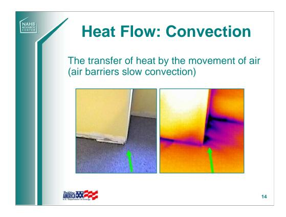
Convection is the transfer of heat by the movement of a fluid (air).
