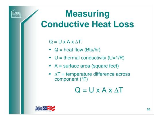
The energy loss through a material (e.g., wall or building envelope) is directly proportional to its surface area, U value, and the temperature difference across the material.
