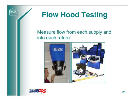
Another approach to measuring duct system performance is to measure the flows into and out of the grilles, add the supply air and return air separately, and compare this to what the intended system flow. The device used for this test is called a flow hood.
