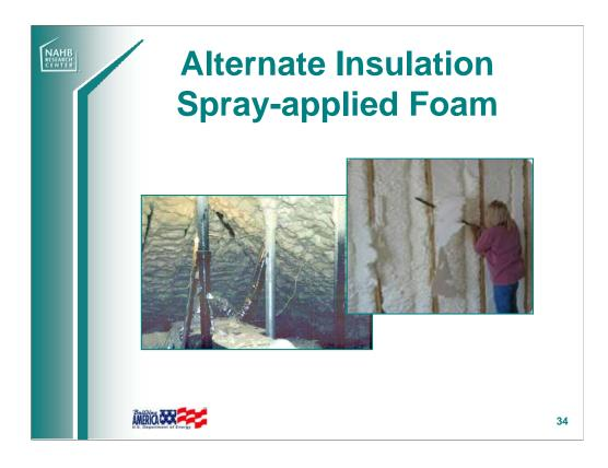
Spray applied foam provides air sealing as well as insulation. While more costly to install, the results can be dramatic, particularly in finished attics. Another benefit to spray foam is sound reduction. Spray applied insulation is the most effective way to insulate the floor over an unconditioned crawl or basement.
