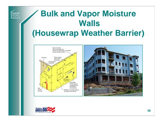
Housewrap can assist in bulk and vapor moisture control in walls. Just like Gore-Tex jackets, it prevents rain from passing through, but allows water vapor to escape.
