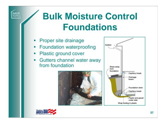
Site drainage, foundation waterproofing, and channeling water away are key strategies in foundation moisture control.
