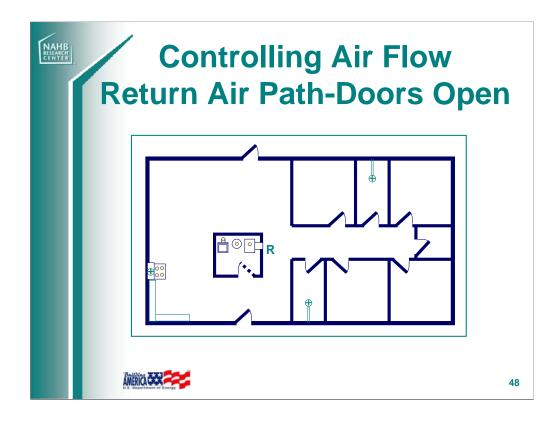
In a house with central returns, the return air pathway is critical to maintain balanced interior pressures.
