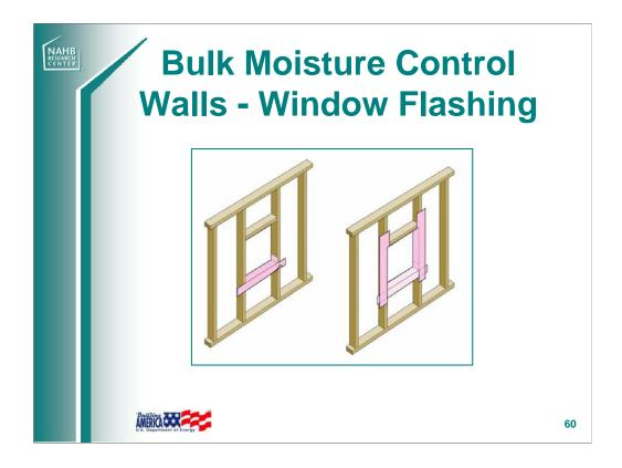
When installing windows, a flashing system must integrate the housewrap or felt with the window opening.
