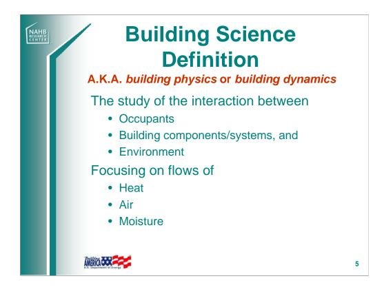
Building science is the study of the interaction between occupants, building components/systems, and the surrounding environment. It focuses on the flows of heat, air, and moisture.
