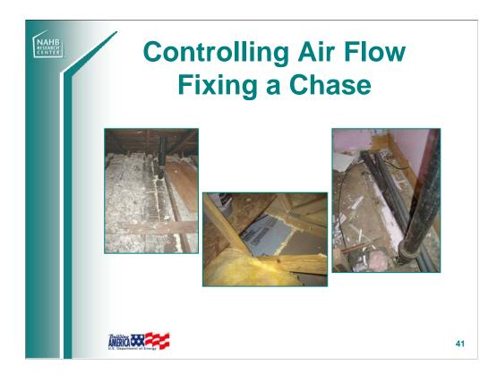
Chases carry conditioned air out of the house as a result of the stack effect, fan-driven pressure imbalances in the home, and wind.
