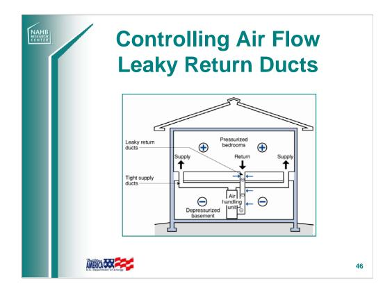
Pressure imbalances can drive air leakage, with air leakage increasing as the pressure differences increase.
