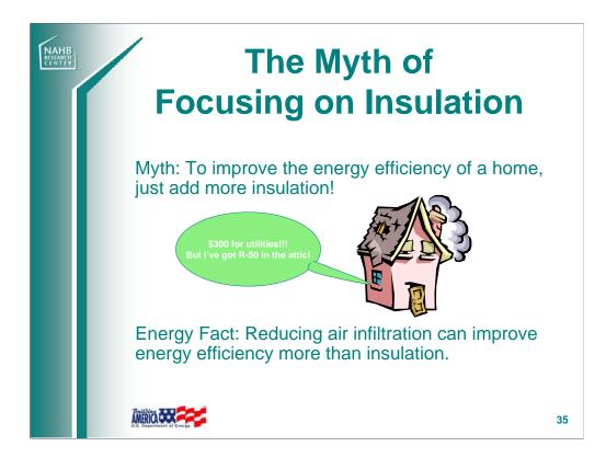
Focusing on insulation alone to improve energy efficiency can be short sighted.
