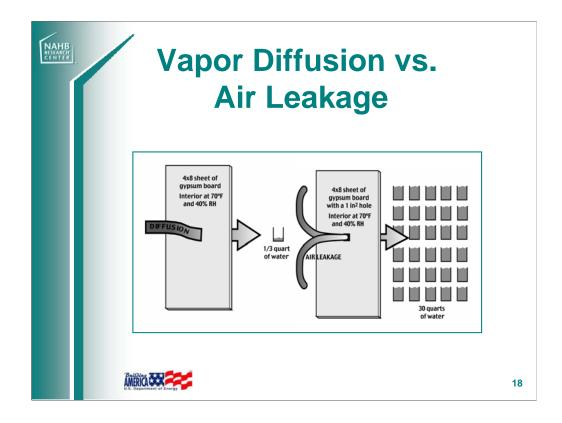
Air leakage is the primary way in which water vapor enters a home. Air coming into (or out of) a home carries a lot of water vapor with it. Infiltration has a much greater impact than vapor diffusion (transport of water vapor through a material) on the amount of moisture entering a home.
