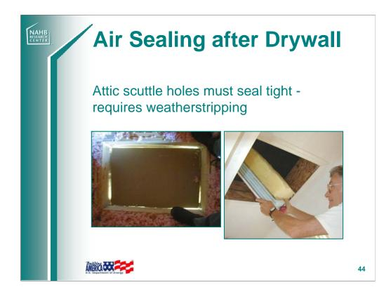
Attic scuttles can become a "big gaping hole" in a home's envelope if not treated appropriately, especially since they are located at the top of a house, which is usually at the highest pressure due to the stack effect.
