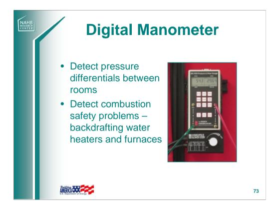
Manometer is part of the blower door and duct blaster setups, but can be used alone to diagnose pressure differences between rooms and zones of a house.
