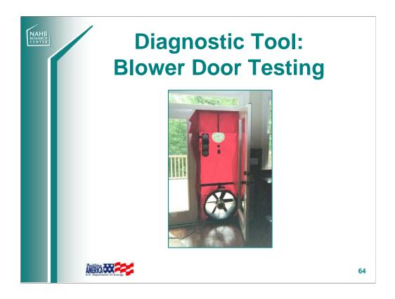
A blower door is a device that is installed in an exterior door and has a calibrated fan that can quantify air leakage in a home.
