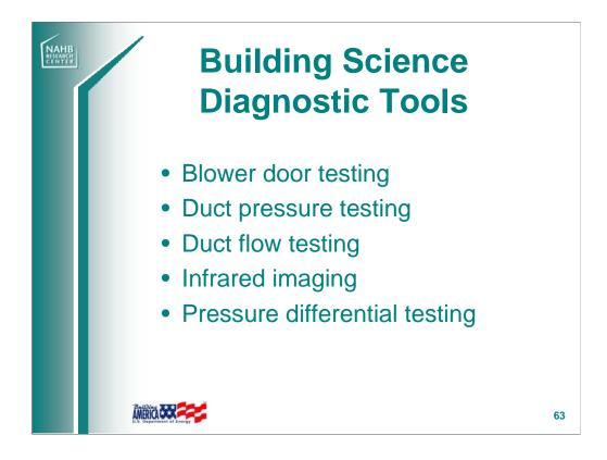
There are a number of diagnostic tools available to help you understand how a home performs and why. Diagnostic testing also can confirm the effectiveness of improvement work such as duct sealing. Diagnostic testing frequently surprises many conscientious heating and cooling contractors when it shows that their systems are leakier than they had assumed.
