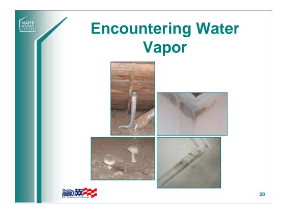
Water vapor is usually noticed in homes when building surfaces cool below the air's dew point, causing the water vapor to condense on the cool surface. This moisture can cause mold and fungus deterioration. In addition, high interior humidity in the warm summer months can make a home feel uncomfortable and cause occupants to lower thermostat settings to achieve the same level of comfort.
