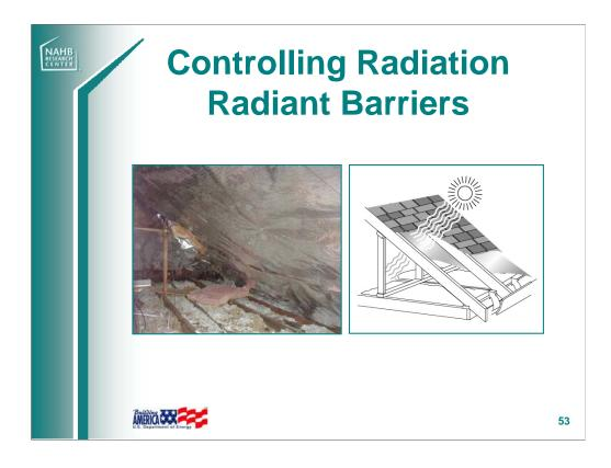
Radiant barriers are reflective materials that can reduce summer heat gain in attics. They can also reduce heat loss (see basement photo with foil faced insulation sheathing). They are particularly effective in homes in cooling-dominated climates where cooling equipment and ductwork is contained in the attic.
