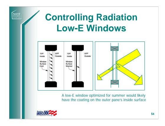
Low-E glazing in windows can significantly lower the heat gained or lost through windows. Solar Heat Gain Coefficient is a number between 0 and 1 that indicates the amount of solar radiation that passes through the window as heat.
