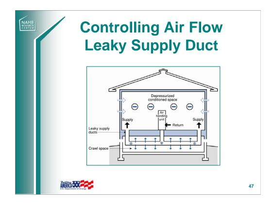
Leaky supply ducts can induce infiltration when the fan is operating.
