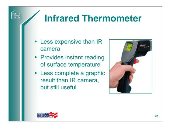
Infrared thermometers can be used to locate heat flow problems in house envelopes and ductwork.
