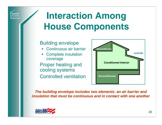
The interaction of the building envelope, heating and cooling systems, and ventilation impact house performance.
