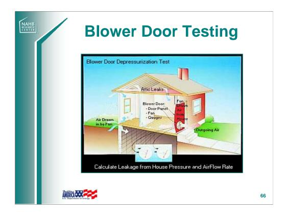
Schematic drawing of a blower door test.
