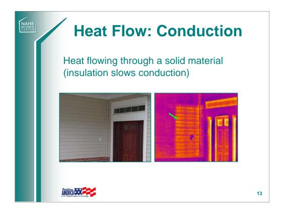
Conduction is heat flowing through a solid material.
