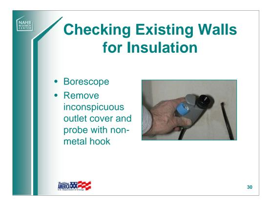
Because wall cavities are typically concealed, various methods to determine insulation levels are needed.
