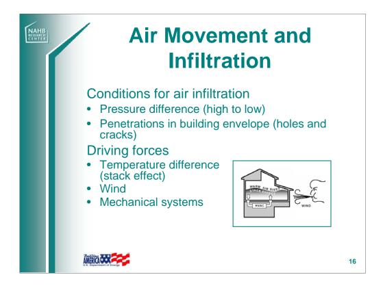
For air movement into or out of a house, two conditions must be present: a pressure difference (air moves from higher to lower pressure) and a hole or other penetration. The amount of air movement depends directly on the pressure difference and the size of the opening.
