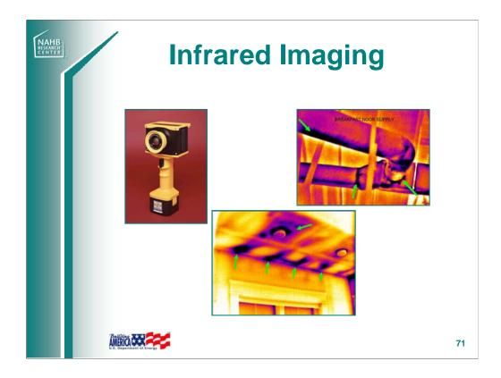
IR cameras can detect temperature differences and show this graphically like a photo, with temperature differences displayed with color.
