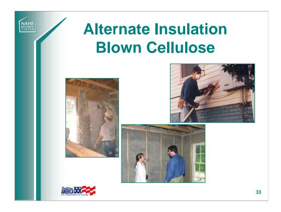
Blown insulation helps to eliminate the problems that can be associated with batts – compression, voids, missing batts. Both cellulose and fiberglass can be blown into wall cavities.
