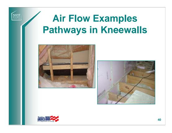
Kneewalls are often overlooked as sources of air flow in the house. However, they often connect many areas of the house. Sealing kneewalls completely can significantly reduce overall air leakage.
