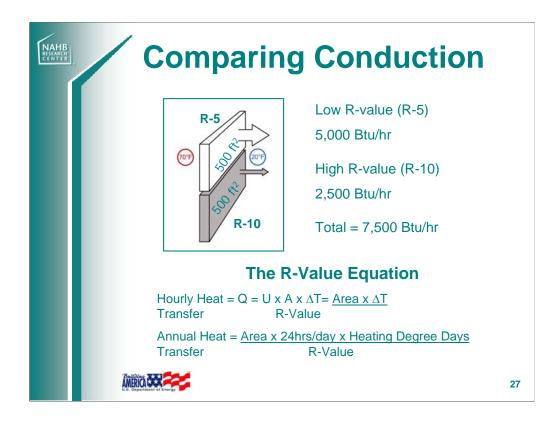
Calculate conduction heat loss through a wall section
