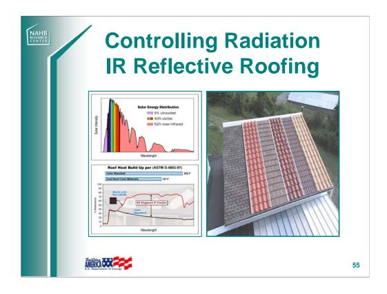
In hot climates infrared (IR) reflective roofing can dramatically lower roof and attic temperatures and, therefore, the house's cooling load and utility costs.
