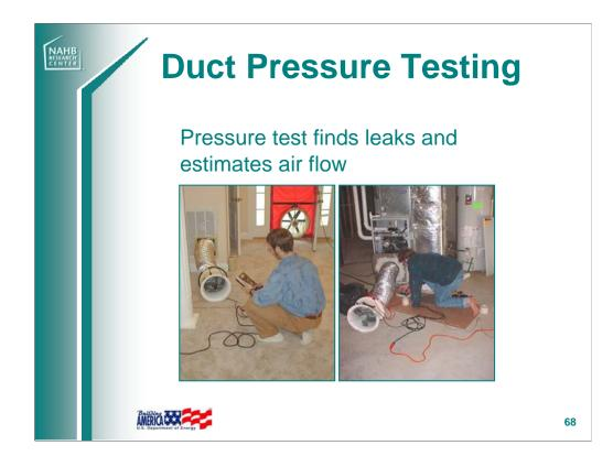
Duct leakage is also a significant source of energy loss in homes when the ducts are located outside the conditioned space such as in attics or basements or crawls. Duct leakage can also enhance house air leakage.
