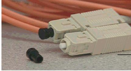
Figure 23. Fiber optic cables with SC connectors
