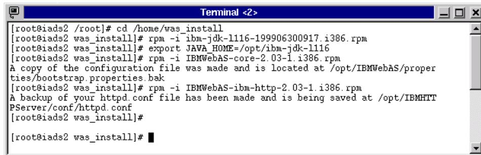
A terminal window titled "Terminal <2>" showing the execution of four rpm commands to install WebSphere components. The output shows the installation progress and messages about configuration files being created or backed up.
