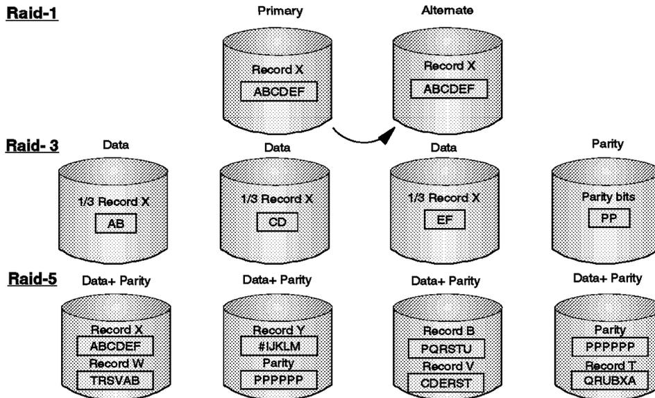
Figure 14. Redundant array of independent disks (RAID)
