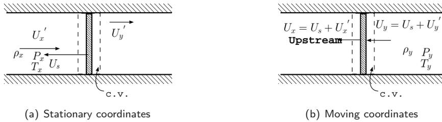
Fig. -6.20. A shock as a result of a sudden and partially a valve closing or a narrowing the passage to the flow
