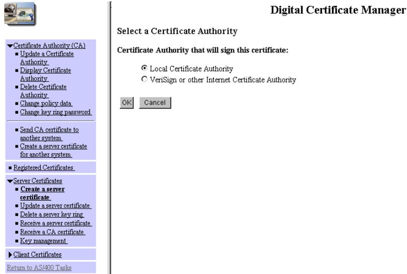
Figure 256. Create a Server Certificate with an Existing Intranet CA
