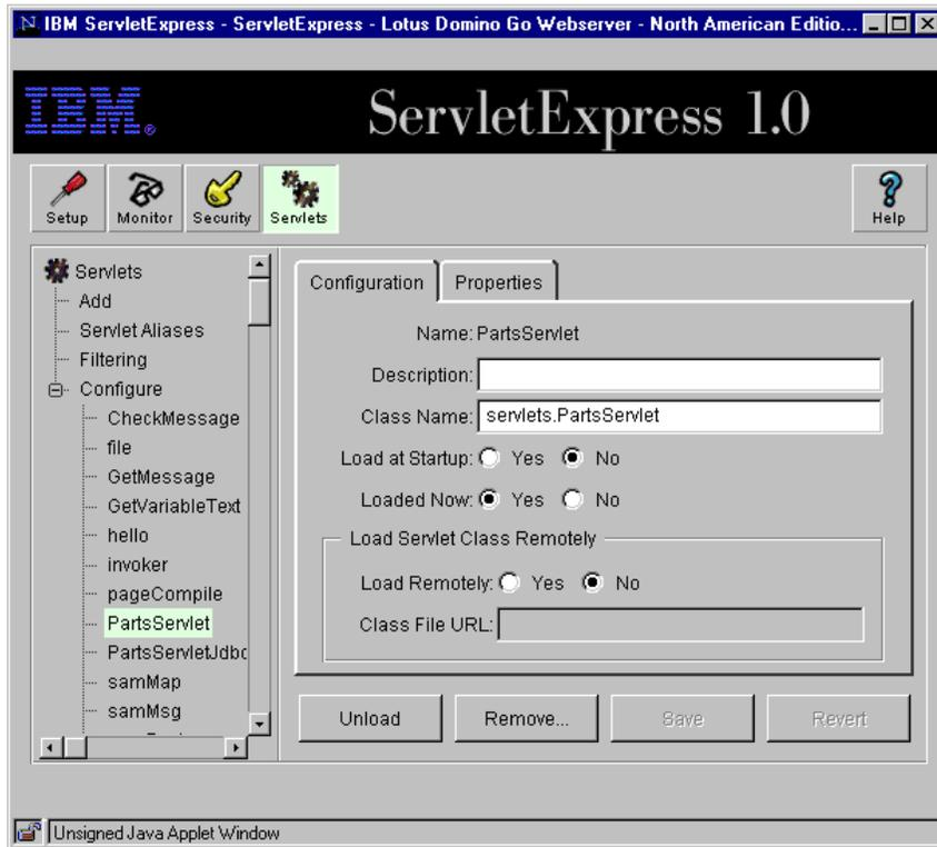
Figure 278. ServletExpress Servlet Configuration Dialog
